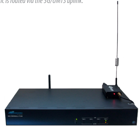
The Barracuda 3G/UMTS Modem M10 attached to a Barracuda NG Firewall Model F101
